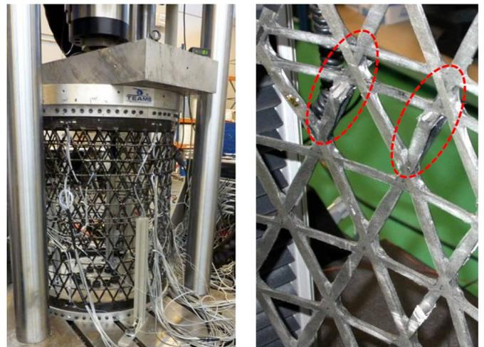
Figure 8. Isogrid structure under compression test. Detail of broken bars after exceeding the max. load
