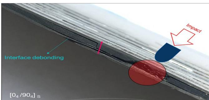
**Figure 5.** Delamination caused at a ( $0_4, 90_4$ )<sub>s</sub> CFRP laminate after a 5 J on-edge impact
