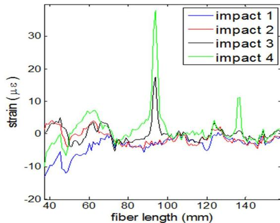
**Figure 6.** Strains recorded by the optical fiber after successive impacts of increasing energy, from 2 to 5 joules. The two identifiable peaks recorded at 100 and 140 mm are for the first and second loops of the optical fiber, respectively
