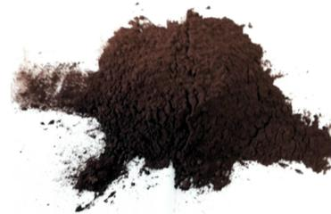
**Figure 2:** Kraft lignin as a brown fine powder after drying.
