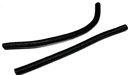
**Figure 7:** Lignin:PHB blend for 75:25 extruded with the 3 mm die.
