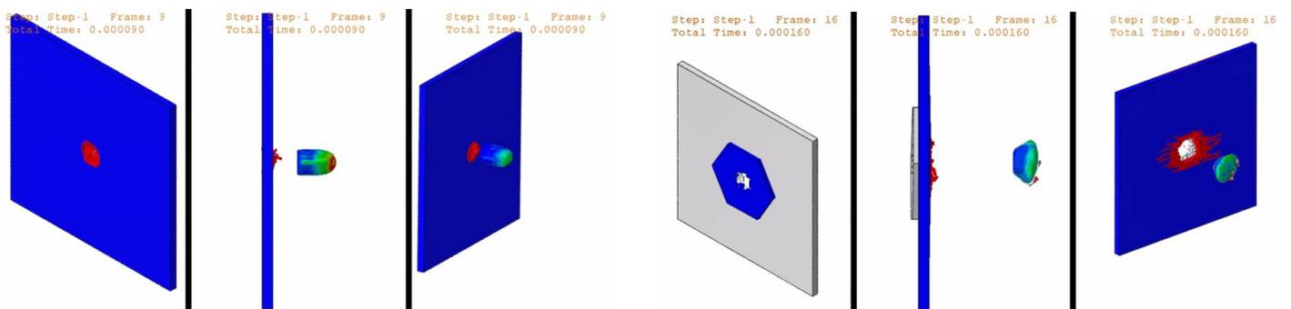
**Figure 3.** Numerical model of the bullet penetrating the CFRP, depicting the damage in the HS300/ER563 material and bullet plastic deformation from different angles (entry side – left, side view – middle and exit side - right).
