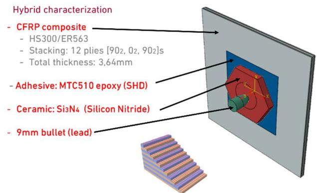
**Figure 2.** Schematic of the target showing the different layers of material and representation of the bullet.
