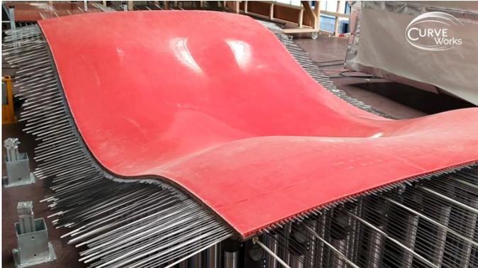
**Figure 2.** Curved mould used by CURVE WORKS as mould for composite manufacturing
